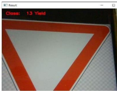
Fig. 9: Yield sign detected through the web cam
