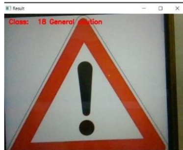
Fig. 11: General Caution sign detected through web cam
