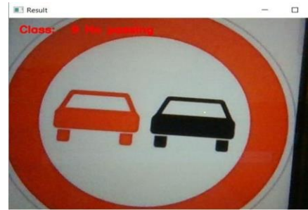
Fig. 10: No Passing sign detected through web cam
