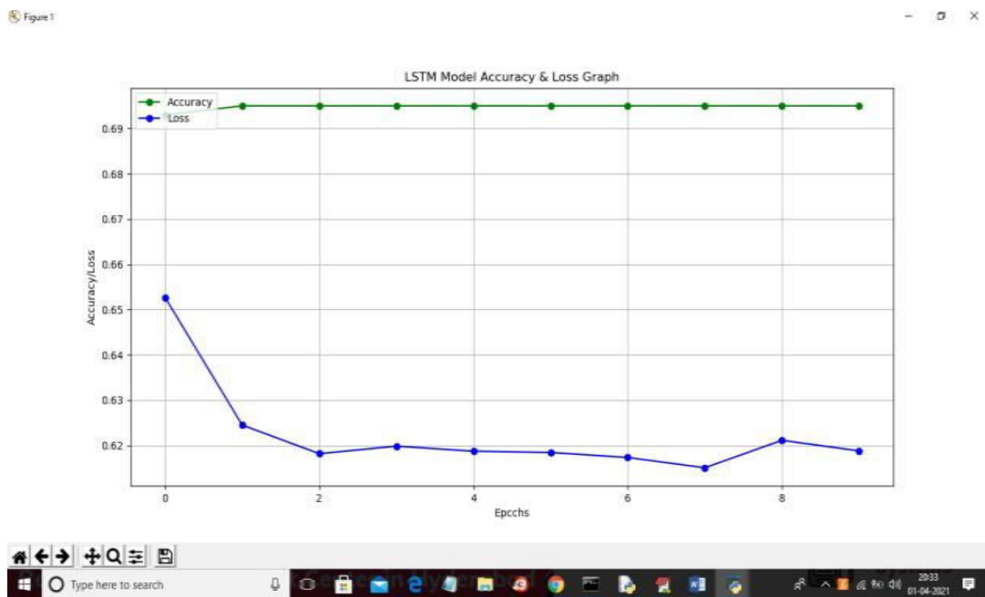
Figure 7. Above, the x-axis stand for epoch/iterations and the y-axis stands for correctness and loss value, with the green line representing correctness and the blue line representing loss value, and with each rising epoch, loss values drop and accuracy reaches 70%.
