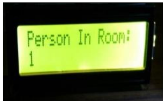
Fig 6: Person enters in the room, LCD shows no. of person 1 & Light is turn OFF
