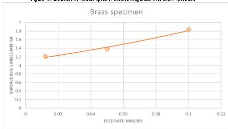
Figure 4.4 Influence of feed rate to surface roughness over Brass specimen
