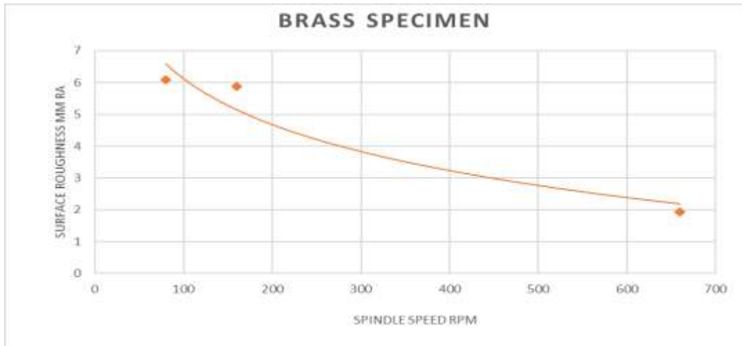
Figure 4.3 Influence of spindle speed to surface roughness over Brass specimen
