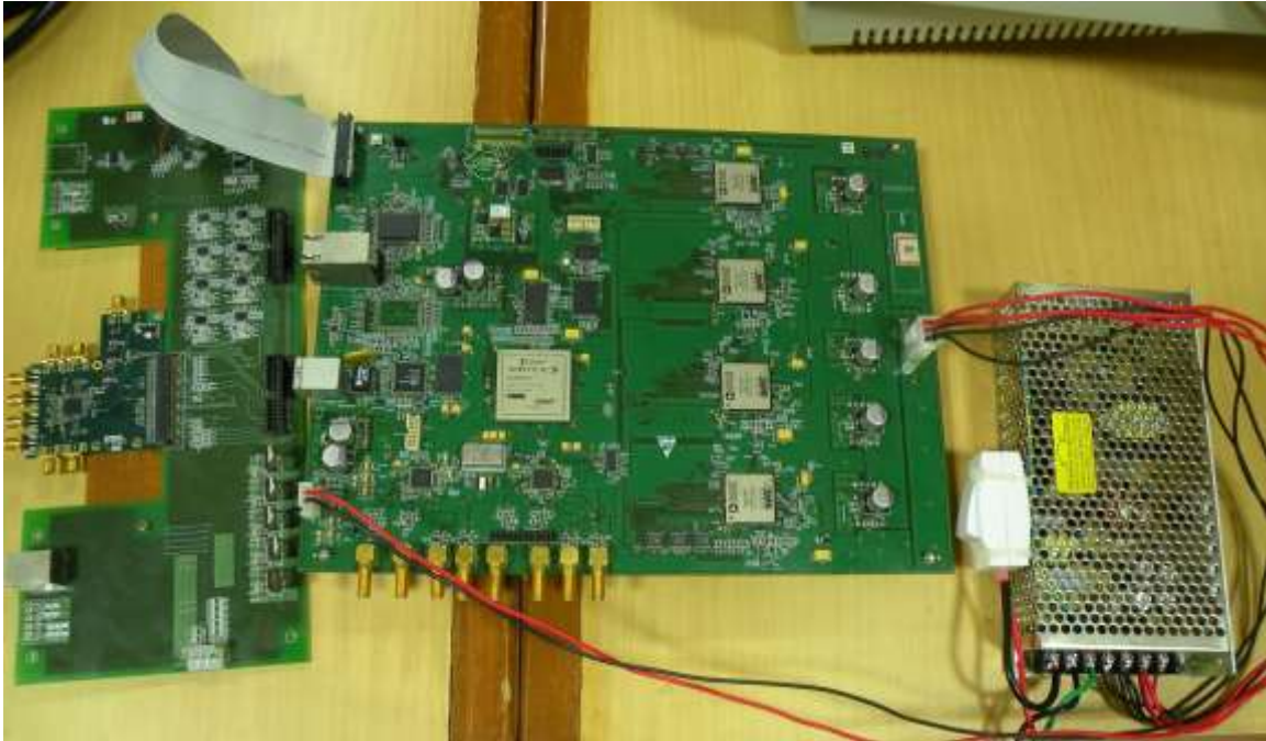
Fig. 3.3: Picture of hardware of the WiMAX base station.
