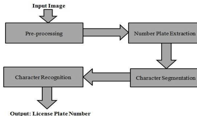
Figure 1: Block Diagram of ANPR.
