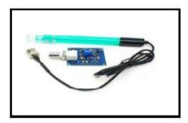
**Turbidity sensor**: Turbidity is a measure of the cloudiness of water. Turbidity has indicated the degree at which the water loses its transparency. It is considered as a good measure of the quality of water. Turbidity blocks out the light needed by submerged aquatic vegetation. It also can raise surface water temperatures above normal because suspended particles near the surface facilitate the absorption of heat from sunlight.
