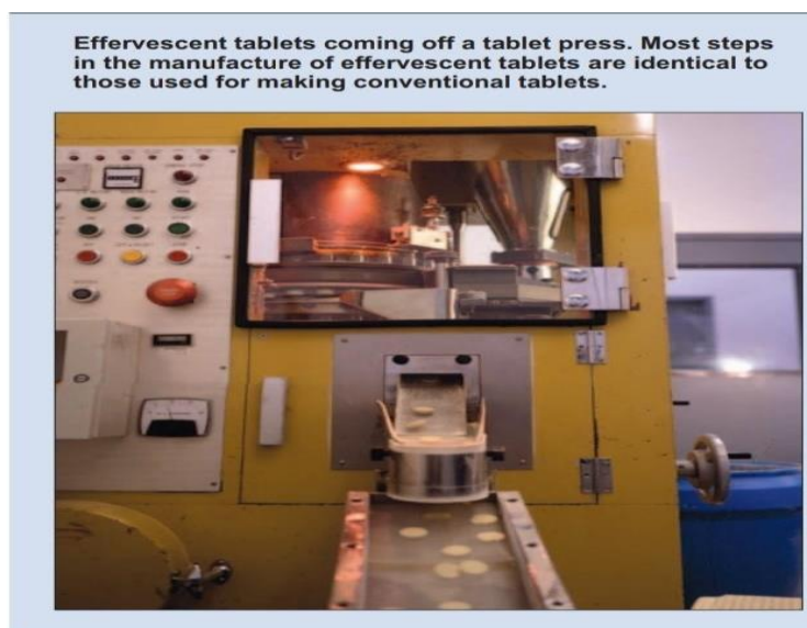
Figure 2: Tablet press making an effervescent tablet.
