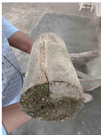
Fig 4: Cross section of a 40% replaced EPS concrete cylinder following a 28-day split tensile test.
