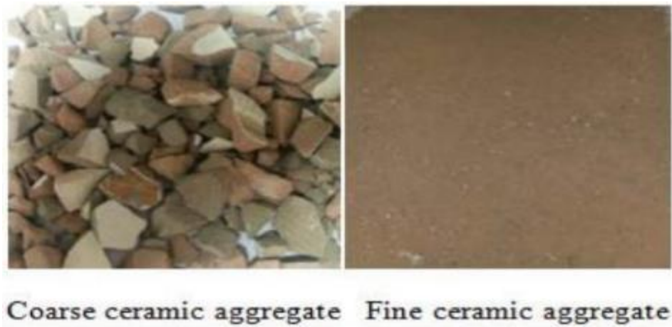
Fig. 2 - : Recycled ceramic tile waste aggregates
