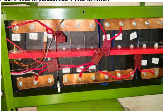
FIG. 9 –Battery pack with 3 cell in parallel and 4cell in series
