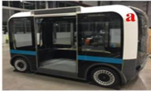
Fig. 4.1 3D Printed Shuttle (Olli) [(Rogers, 2014) Copyrights © Local Motors]
