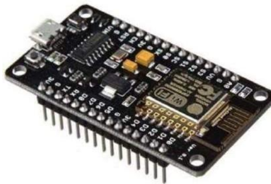
Figure Node MCU ESP8266 Obviously, wire will be used to connect the components.
