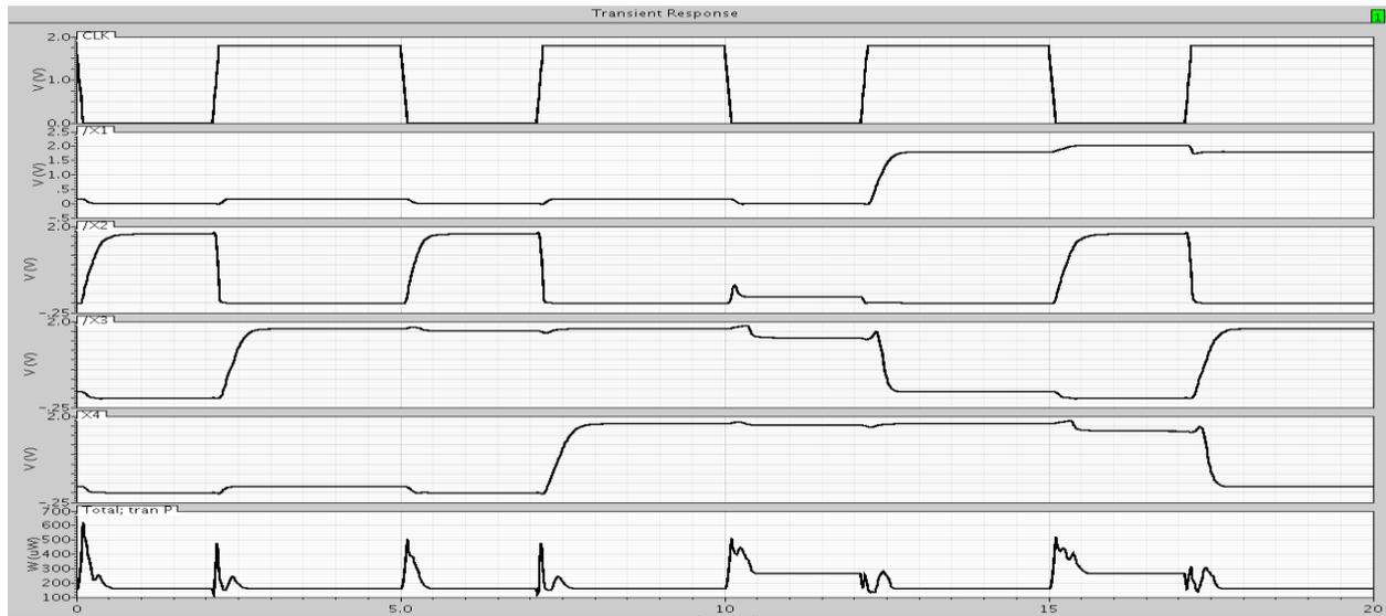
Figure 10. Output wave form at the X1, X2, X3, X4 of LFSR and total power
