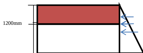
Fig. 3: Earth Pressure on Walls
