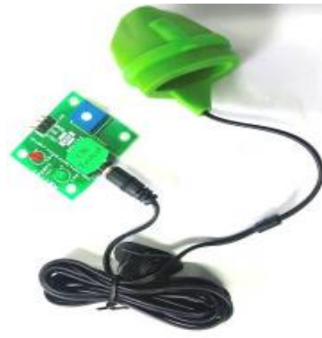
Fig.5 Heart Pulse Sensor with OP-AMP
