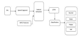
Fig: - System Architecture
