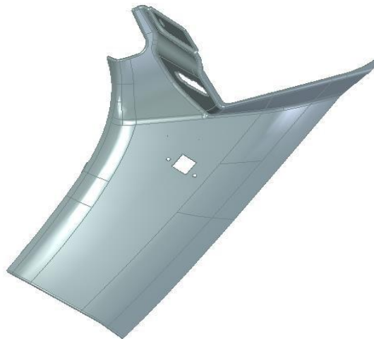
Figure 8: 'C' Pillar after Punching
