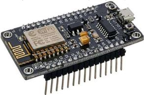
The ESP8266, designed and synthetic through Espresso Systems, consists of all essential factors of the cutting-edge computer: CPU, RAM, networking (Wi-Fi), or even a cutting-edge working machine and SDK. When bought at bulk, the ESP8266 chip expenses simplest three hundred Rs. A piece. That makes it an first rate preference for IOT initiatives of all kinds.
