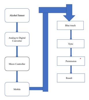
The Block Diagram represents how our project will work. Firstly, when we set the Alcohol sensor it will transfer the signals to Analog to Digital converter (ADC) then this converter converts the analog signal into digital signal and then send to microcontroller after that it will send to the Bluetooth encoder followed by the Bluetooth transmitter finally we will get results in the Android mobile
