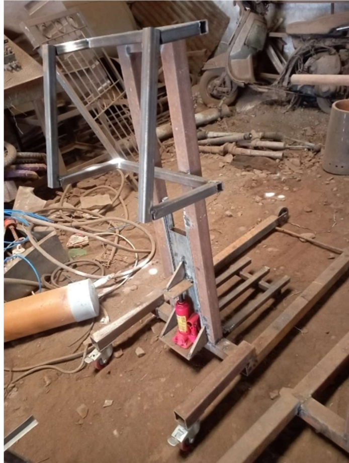
IMAGE OF HYDRAULIC LIFTING CRANE
