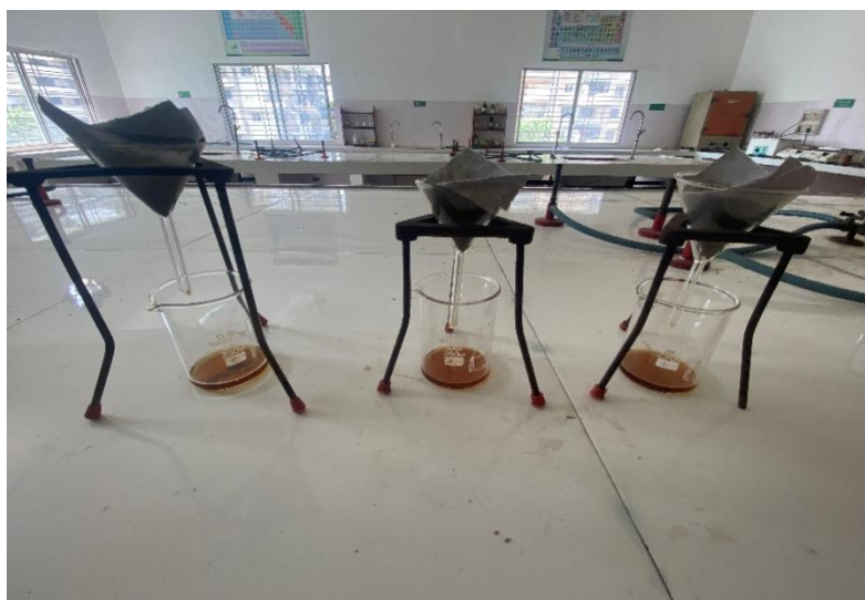
Image No.6 Filtration process in alcohol soluble extractive value
