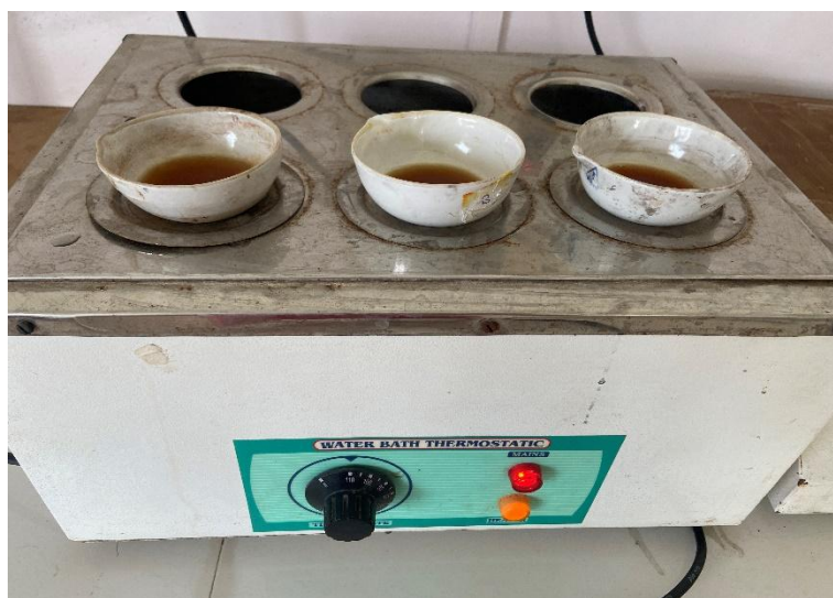
Image No. 7 Filtrate kept on water bath for extraction
