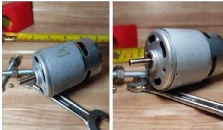
fig 1.2 RS-775 Brushed DC Motor used
