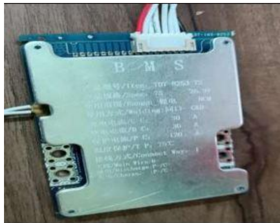
Fig 4 - Battery Management System (BMS)
