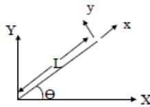
Fig. 3.1 The plane frame element
