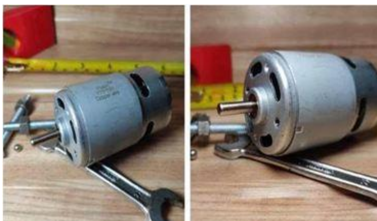
fig 1.2 RS-775 Brushed DC Motor used
