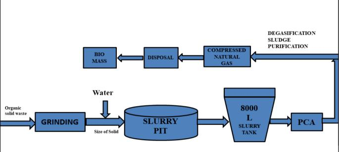
Figure 1- Block Diagram -Slurry Management
