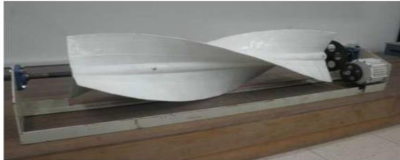
Figure.5 Twisted vertical axis blades
