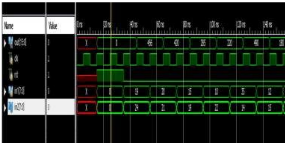
figure 2.9. Simulation result of RNS multiplier using Ladner Fischer parallel prefix adder.
