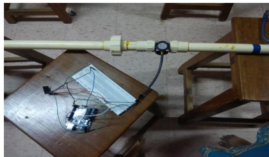
Figure 4.3 Fixing of water flow sensor
