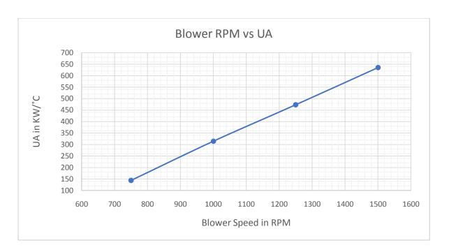
The test is conducted to investigate effect of blower speed on overall heat transfer coefficient (UA) of system. The overall heat transfer coefficient is calculated by equation no. 3.2 and 3.3 in data reduction, it is found that the overall heat transfer coefficient increases with increase in blower speed. This is due to increase in mass flow rate.
