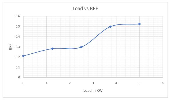
The test is conducted to investigate effect of load on bypass factor of system. The bypass factor is calculated by equation no. 3.1 in data reduction, it is found that the bypass factor is increases with increase in load in system. It is seen from the graph that bypass factor drastically increases from 2.5 KW and is maximum at 5 KW load.
