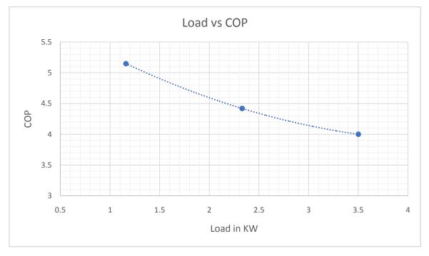
Partial load tests conducted for RAC showed that as the load decreased, the COP increased and the highest COP was obtained at around 30%–50% load; as the load decreased further, the COP decreased.
