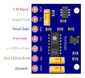
The MAX30100 is a multi-function sensor used in many applications. It is a heartbeat monitor and pulse oximeter. The sensor consists of two Light Emitting Diodes, a scanner, and a series of low-frequency signal processing devices to detect heart rate and pulse oximetry.
