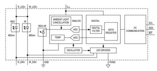
The output from the photodiode is sent to an analog-to-digital converter where digital data is sent from the filter to the digital data register. Data can be collected from the register and can be sent to a sub-directory via the I2C communication protocol.
