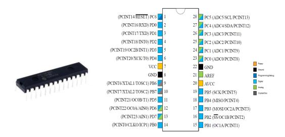
ATMEGA328P (ARDUINO) is a small controller from the 'AARDUINO (ATMEGA328P) 16F' family and developed by MICROCHIP TECHNOLOGY. It is an 8-Bit CMOS Microcontroller with nano-Watt technology. This little controller is popular among hobbyists and engineers because of its features and cost.
