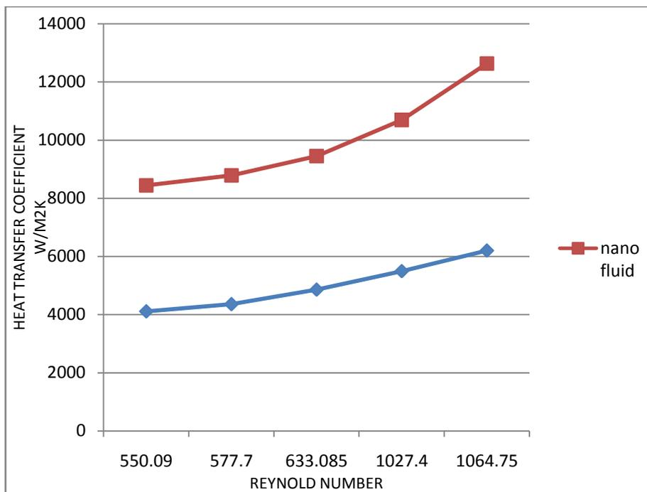
Fig.3.Variation of Heat transfer coefficient with Reynolds number
