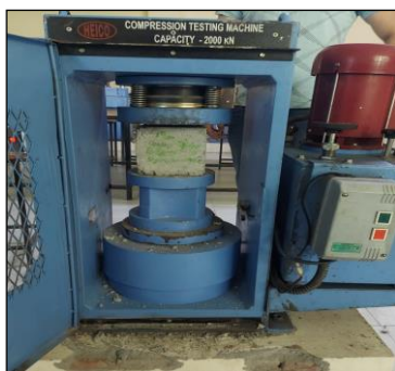
Fig; compressive strength check of block.
