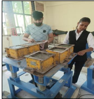
Fig; Mould filling.
