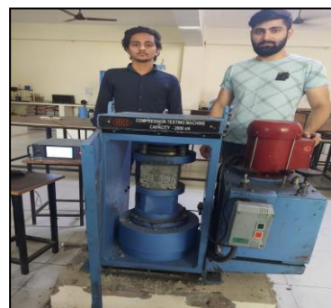
Fig; compressive strength check of block.
