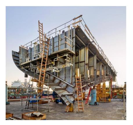
• The panels are then converted into blocks. Blocks are the shape which is achieved by curving the panels and then making them to hold tons of load for a long period of time.
