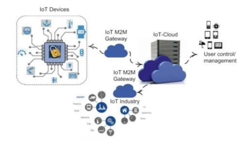
• This is how the M2M technology works, it takes the data from the working devices then stores them in the cloud and then continuously uses the data to improve user experience.
