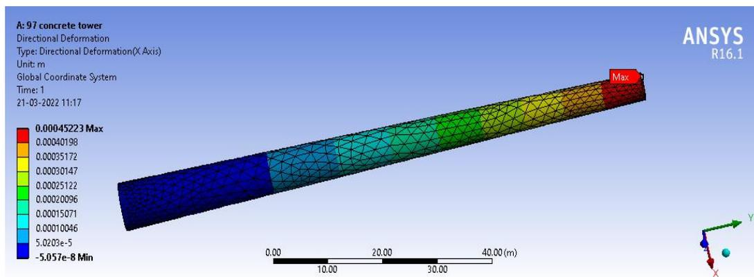
Figure 6 Contour of directional deformation for concrete material
