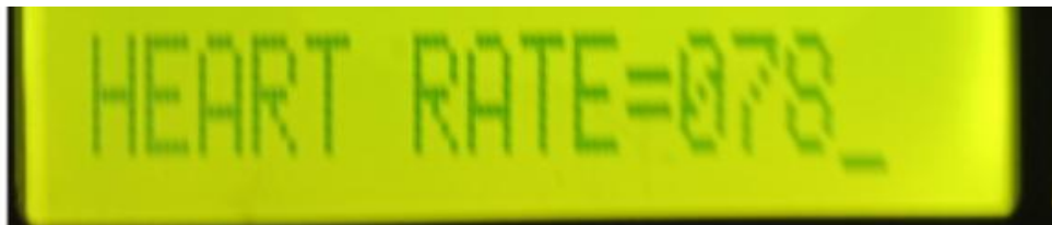
LCD SCREEN SHOWING HEART RATE OF BODY BY PULSE SENSOR
