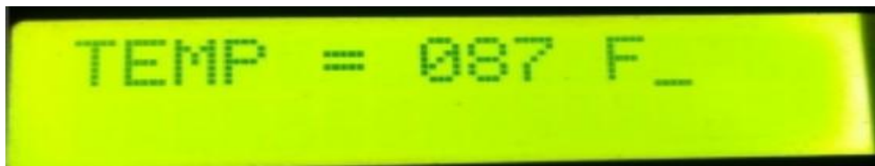
LCD SCREEN SHOWING TEMPERATURE OF BODY BY LM-35
