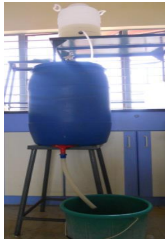
Figure 2: Experimental Set Up of Vermifiltration Kit
