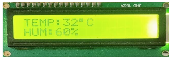
Fig 4-Temperature and Humidity at normal level
