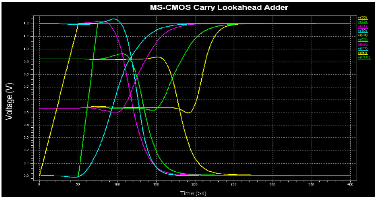
Figure 10: Sum and carry signal transitions for 4-bit MS-CMOS Carry Lookahead Adder
