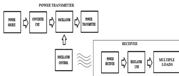
In the transmitter section the step down motor is used. The motor is reduced the primary voltage. Its affair is given to regulated power force. The regulated power force is used to convert the AC 230voltage to 9VDC regulating voltage. ThisDC voltage is given to the resonator.
