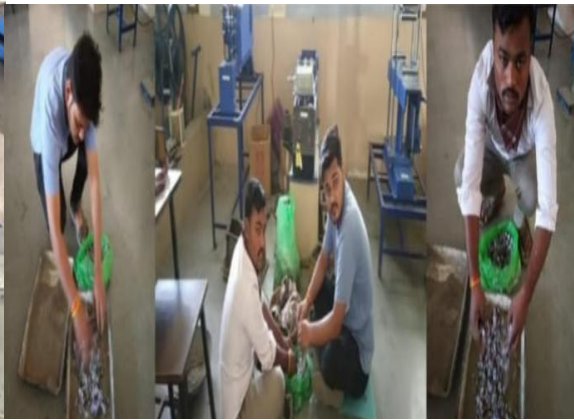
Fig. 5 Adding paperpulp to concrete mixture
