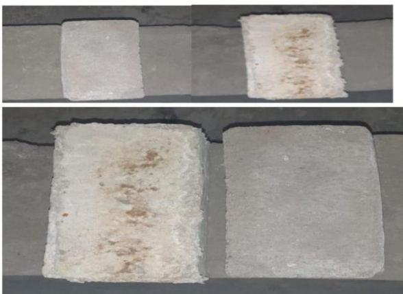
Fig. 6 Concrete bricks after 7 and 28 days curing
