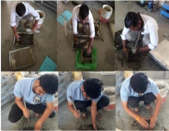
Fig. 4 Preparation of Concrete brick mixture
