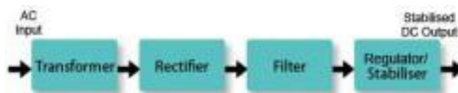
Figure 7: Block diagram of a fixed regulated power supply
