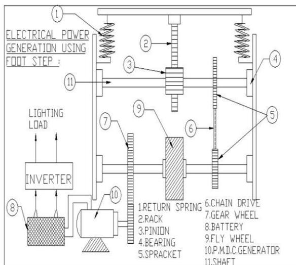
When the force is released from the plate, the pinion reverses and moves another circle, causing rotation of gear pairs.
