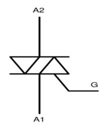
A TRIAC is bidirectional thyristor with three terminals. It is used significantly for the control of electricity in ac circuits. TRIAC is the phrase derived by using combining TRIODE and AC. Basically it is a switchingdevice.
