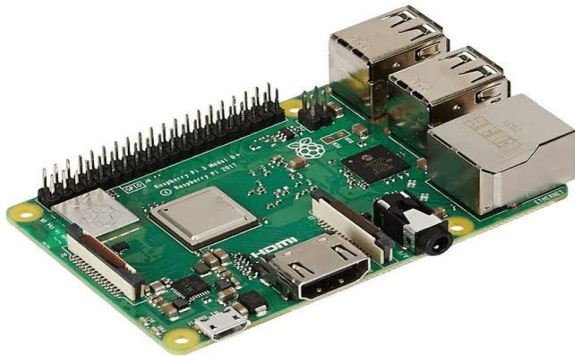
Fig. 1: Raspberry pi 3B+
