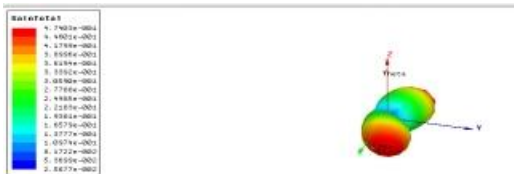
Fig 9: Gain of SRR-Slot at Upper C Shaped
