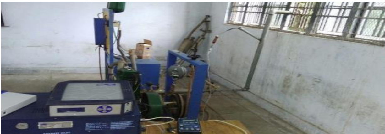
Figure5 Exhaust gas analyzer probe connected to exhaust.
