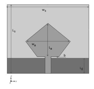
The design and implementation of a pentagon antenna for brain cancer and stroke detection, positioned directly on human's head. It is simulated using HFSS software that is High Frequency Structure Stimulator Software and fabricated on FR-4 substrate with relative permittivity 4.4 and thickness 1.5mm. The HFSS antenna gives theresult in 3D format. It mainly used with the products like antennas, antenna arrays, printed circuit board etc...
