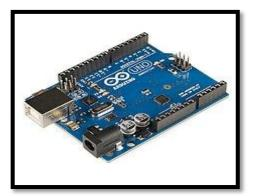
though it accepts voltages between 7 and 20 volts. It is also similar to the Arduino Nano and Leonardo. The hardware reference design is distributed under a Creative Commons Attribution Share-Alike 2.5 license and is available on the Arduino website. Layout and production files for some versions of the hardware are also available.
