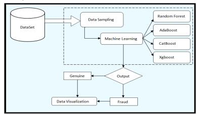
This system consists of four algorithms: one for bagging and the other three for boosting.
